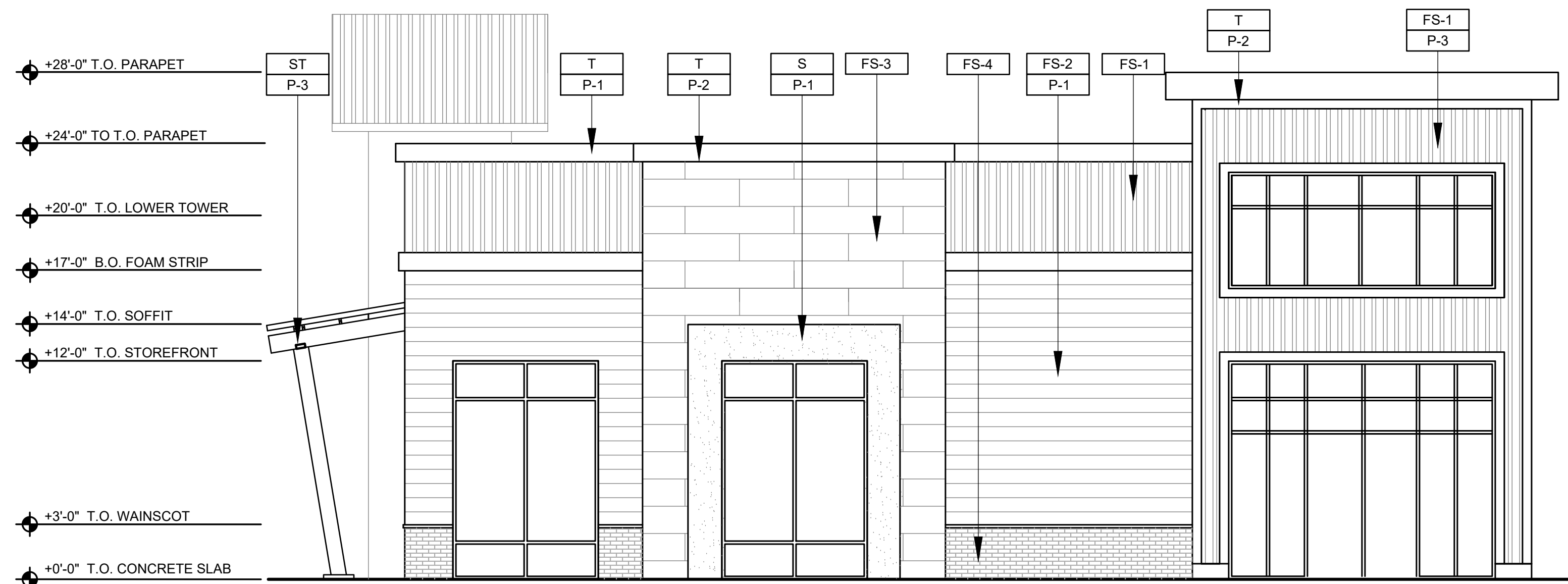
NORTH ELEVATION (SOUTH ELEVATION MIRRORED) 3/16" = 1'-0"
